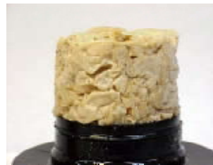
Individual pellet capsules after 50,000 miles of use meld into a single, gelatinous clod blocking the flow of coolant through the filter.
