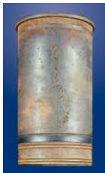
A cylinder liner destroyed by cavitation-erosion
