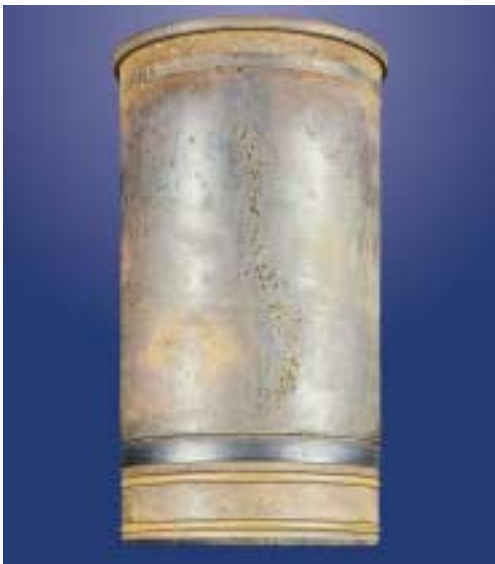
Figure 1 A cylinder liner destroyed by cavitation-erosion.
